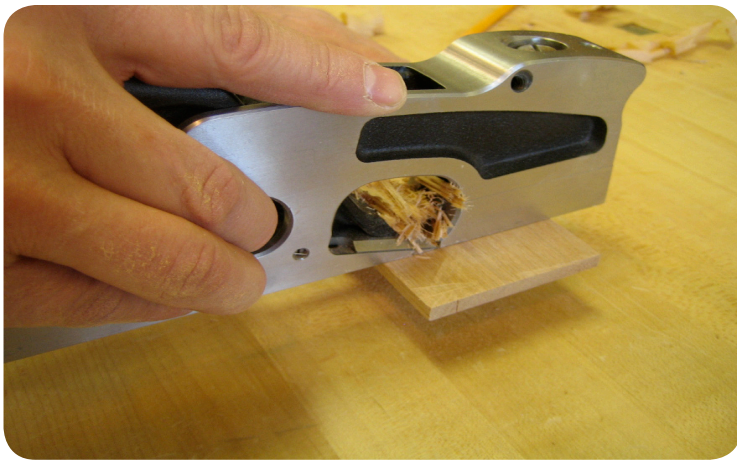
Use a shoulder plane to trim the tenon cheeks to the layout lines.
