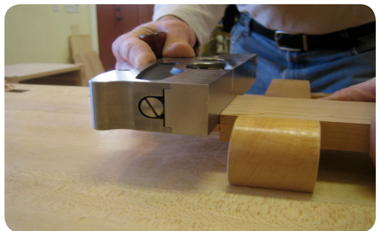
Use a shoulder plane to clean up the tenon shoulders.
